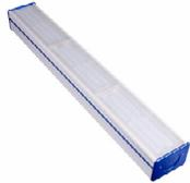
The ELPL-MC-VS3 LED array has a total capacity of 275W (55W blue and UV + 165W of 85% McCree curve + 55W of Red and IR) but is de-rated to 250W to increase LED lifespan. The LED array in each light is dimmable on a channel-by-channel basis, to produce a variable spectrum that can be a close (95+%) match to the McCree curve (depending on user settings).
