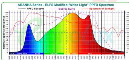
The ARANHA-670 and ARANHA-1000 lights are available with a standard ELFS spectrum which is based on the popular modified 'White Light', good enough full spectrum, with output throughout the PAR range from 400nm to 750nm. This spectrum has a good balance between the ideal spectrum (McCree curve) and cost, with a 70% match to the McCree curve.
